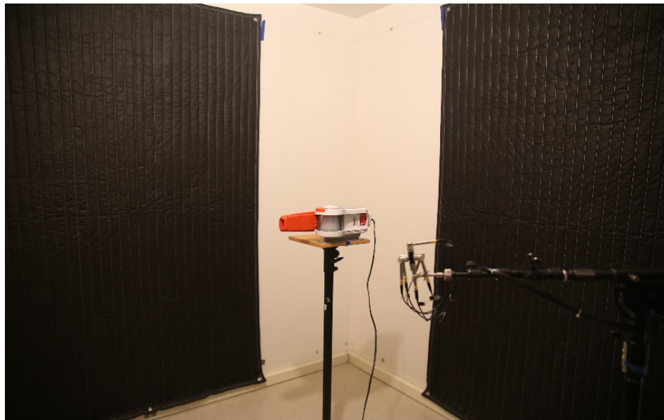
Fig. 4.18. The handheld vacuum in the VAC with the four-blanket configuration.
