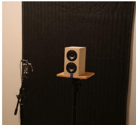
Fig. 4.10. Reference directivity loudspeaker used in the VAC with two blankets and four blankets to study the effects of spatial averaging. The lower cone is the active driver, while the upper cone is a passive radiator.
