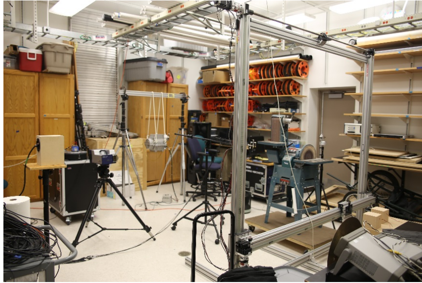
Fig. 4.23. The two-point in situ method in room U186C of the Eyring Science Center on BYU campus. The reference directivity speaker and the belt sander are shown. This room is used for equipment storage and experiments.
