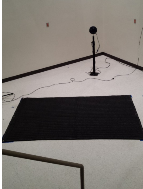
Fig. 4.1. The experimental setup for measuring the absorption coefficients of the blanket in the BYU reverberation chamber. A 20 cm dodecahedron loudspeaker was used as the excitation source and the measurements were taken according to ISO 354.
