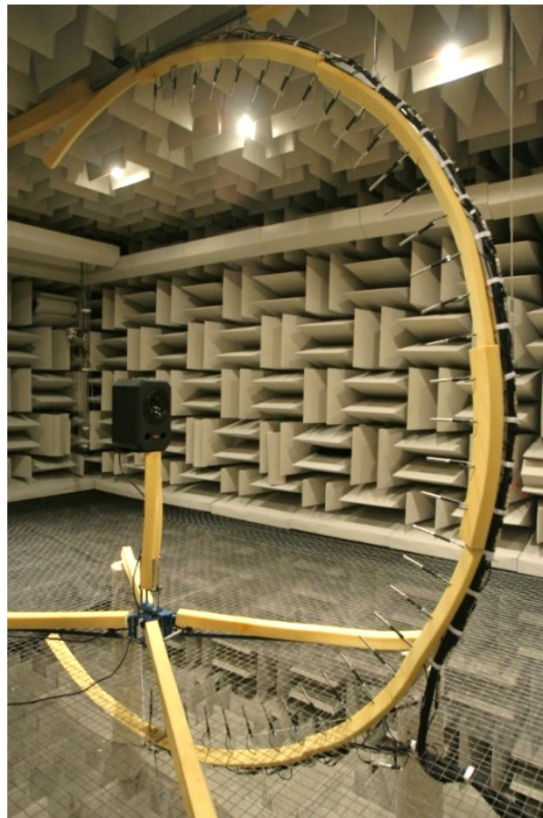
Fig. C.1. Semicircular arc array in the BYU anechoic chamber with a radius of 1.8 meters from the circular center to the microphones. The source sits on a turntable, which rotates it a full 360^\circ in the azimuthal angle.
